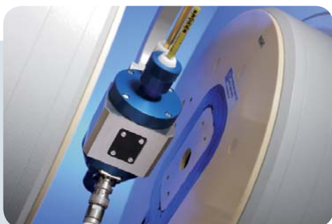
Rapid scan coils mounted on the magnet pole face
