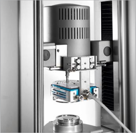
Rear view of the active upper temperature control unit
