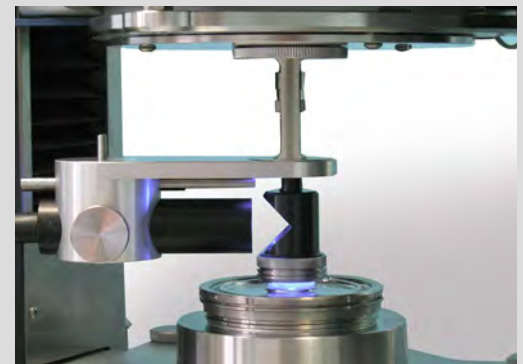
UV curing cell
