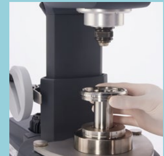
Quick bayonet mountings for short pre- and post-handling time per measurement
