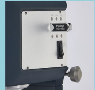
USB memory stick for job and data transfer between instrument and PC
